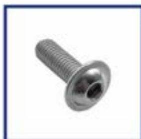
HINA-SCREW006 内六角圆头带垫螺钉 Hex Socket Pan Head Screw ISO7380-2 Size:M4 M5 M6 M8 Material:SS304,SS201, Q195,C1022
